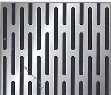
PATTERN No.SL-17520 Diam. 1.75 x 20 mm. Pitch 1 - 4.00 mm. Pitch 2 - 23.50 mm. Open Area 36.53%
