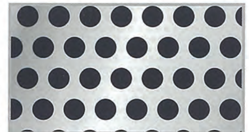
PATTERN No.12 Diam. 5.2 mm. Pitch 7.6 mm. Open Area 42%
