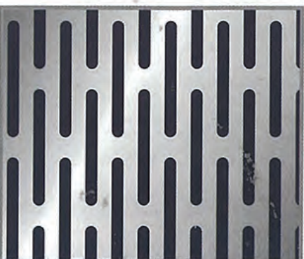
PATTERN No.SL-2020 Diam. 2 x 20 mm. Pitch 1 - 4.50 mm. Pitch 2 - 23.50 mm. Open Area 37%
