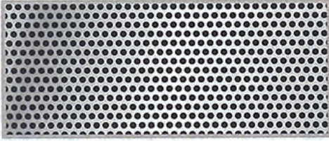
PATTERN No.SKR-11 Diam. 1.1 mm. Pitch 1.6 mm. Open Area 43% Size 300 mm x100 m (Coil)
