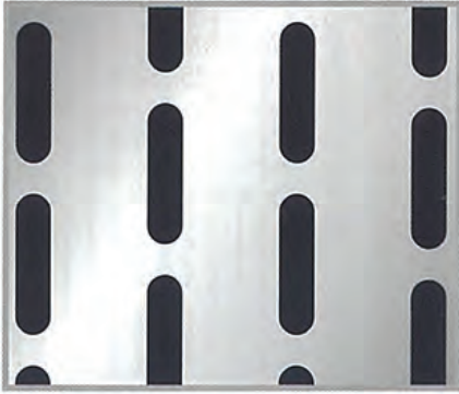
PATTERN No.SL-4016 Diam. 4 x 16 mm. Pitch 1 - 15.00 mm. Pitch 2 - 19.50 mm. Open Area 41.4%
