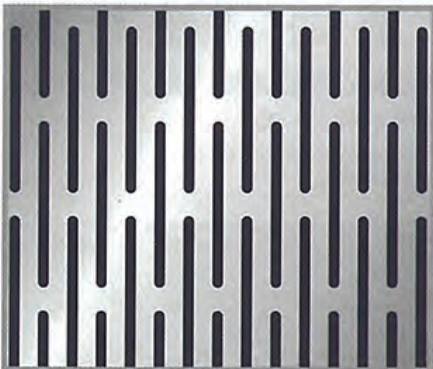
PATTERN No.SL-12520 Diam. 1.25 x 20 mm. Pitch 1 - 3.50 mm. Pitch 2 - 23.50 mm. Open Area 30%
