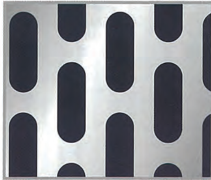
PATTERN No.SL-7020 Diam. 7 x 20 mm. Pitch 1 - 12.00 mm. Pitch 2 - 25.00 mm. Open Area 43.15%
