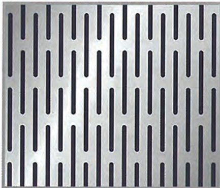
PATTERN No.SL-1015 Diam. 1 x 15 mm. Pitch 1 - 3.00 mm. Pitch 2 - 17.50 mm. Open Area 28.16%
